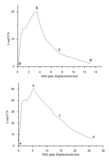
Fig. 3. Load mid span displacement curve of concrete beam: up– $H=50\,{\rm mm},$  bottom– $H=200\,{\rm mm}$
