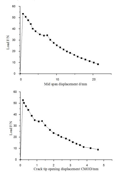
Fig. 1. Load displacement curve and load crack opening displacement curve of concrete beam specimen: upper part–load displacement curve, bottom part–load crack opening displacement curve
